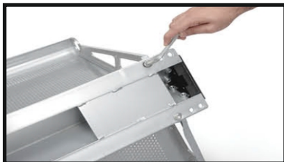
Step 2: Fasten the beam with allen keys
